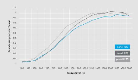
α<sub>w</sub>-value: 0.55 (MH), standard absorbent, class D (19.5 kPa s/m²)
