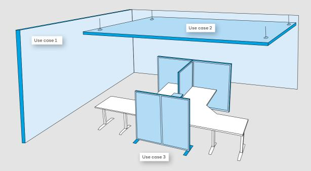
A room's acoustic quality is also influenced by its geometry, the selection and distribution of sound-absorbing and sound-reflecting surfaces, as well as by reverberation time and noise.
